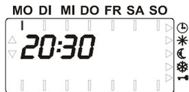
The clock can be set once the
