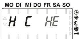
When you press the **PROG** program button for 6 seconds, you are taken to a menu where various basic functions can be set. The functions are shown on the left-hand side of the display and the corresponding value or status on the right.
