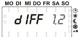
When you press the **PROG** program button for 6 seconds, you are taken to a menu where various basic functions can be set. The functions are shown on the left-hand side of the display and the corresponding value or status on the right.
