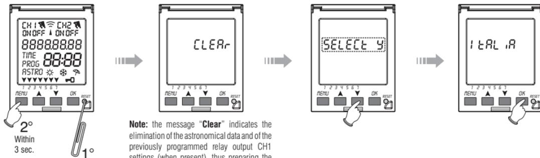
**Note:** the message “Clear” indicates the elimination of the astronomical data and of the previously programmed relay output CH1 settings (when present), thus preparing the appliance for a new programming (the present data are those by default).
