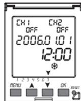
In case there is no mains voltage, the appliance stores the programmed data in its memory and disables the relays. The date and time display will start flashing and after approx. 2 minutes the display will switch off (stand-by mode).
