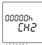
**Note: the timer does not move forward if the instrument is not connected to the power supply**
