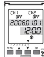
This time switch is supplied in idle state (SLEEP-MODE) to avoid unnecessary battery consumption.
