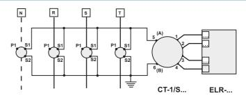
CT1S: It's a summation T/T, which should be used, in those cases when the cables of the system to be protected are bigger than the inner diameter of the T/T's. In such a case Ct's should be used and installed in the line. The CT's are connected to the summation T/T's and these to the ELR. (For more information, please refer to the applications notes described hereinafter).
